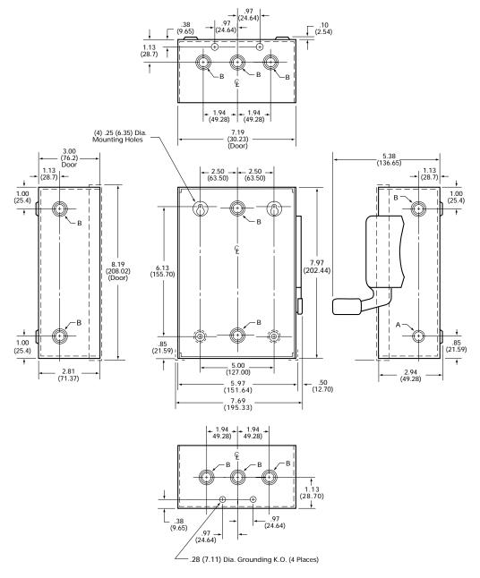
Dimensions shown in inches and millimeters ( ). Dimension shown accurate to  $\pm\,\%$  inch. Note: Handle shown on front and right hand views only.
