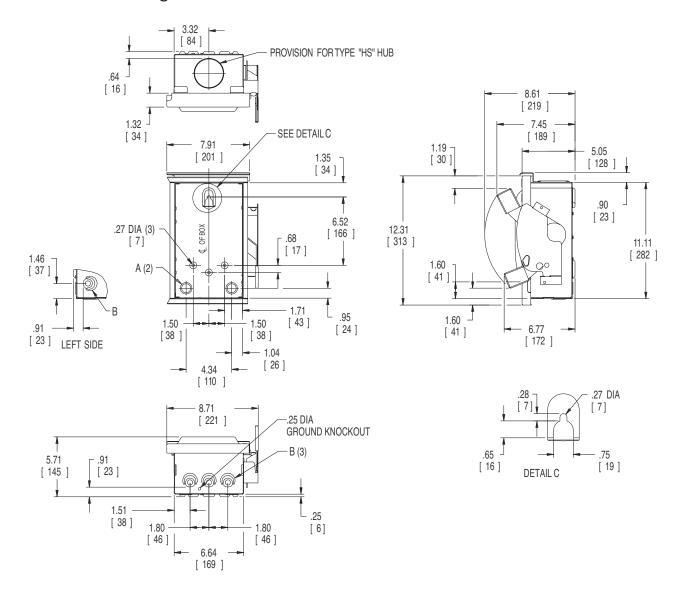
Dimensions shown in inches and millimeters ( ). Dimension shown accurate to  $\pm\,1\!\%$  inch.
