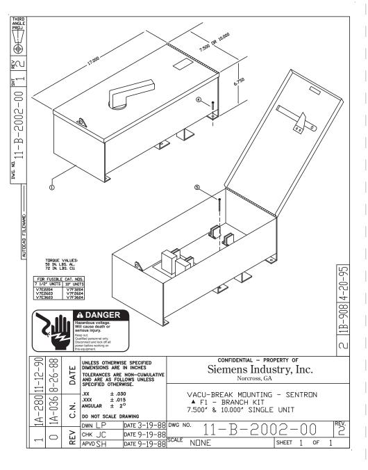
FOR USE WITH 10" HIGH SINGLE UNITS MOUNTED IN SPP/FPP/S4/F1/P4 PANELBOARDS (SHALLOW BOX).
