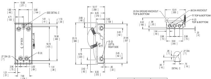
Dimensions shown in inches and millimeters ( ). Dimension shown accurate to  $\pm$  1/8 inch.
