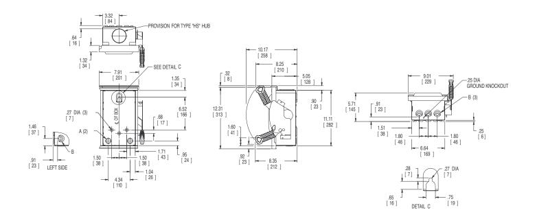
Dimensions shown in inches and millimeters ( ). Dimension shown accurate to  $\pm$  ½ inch.
