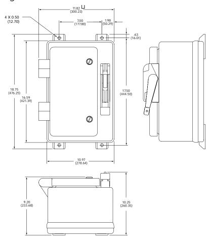
Dimensions shown in inches and millimeters ( ). Dimension shown accurate to  $\pm\,1\!\%$  inch.
