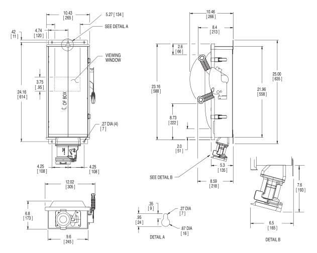
No knockouts in the enclosure. Dimensions shown in inches and millimeters ( ). Dimension shown accurate to  $\pm\,\%$  inch.
