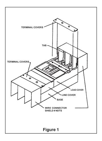
To install catalog #NDTS on MD, ND, MM & NM breakers, motor circuit interrupters and molded case switches
